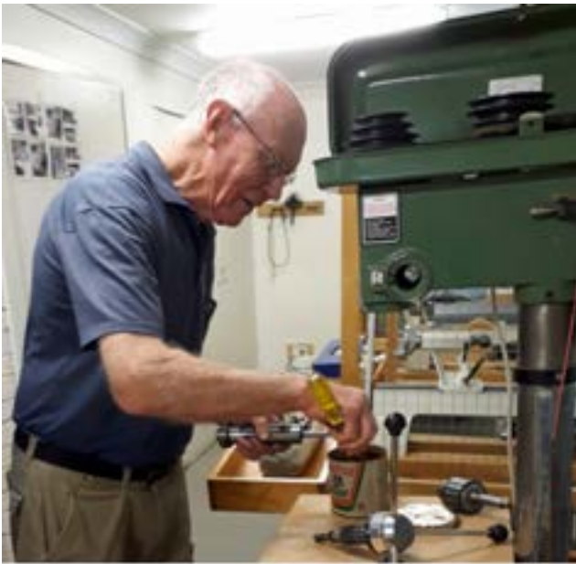
Allan Game Replacing Spindle Bearings in Drill Press
