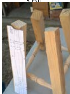
The holes for stretchers are bored before turning
